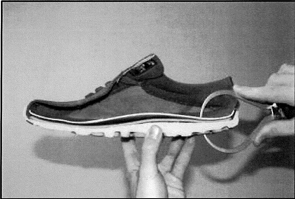
Fig B-2. The caliper must be placed at the middle of the heel when looking from the side
